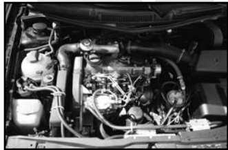
Dual-tank, diesel "Greasecar"; converted by using a system purchased through www.greasecar.com
